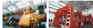
实物轮轴试验台 Full-scale wheelset test stand 24通道电液伺服疲劳试验台 24-channel Electro-hydraulic service fatigue test stand
