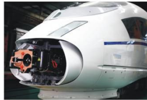
高速动车组全自动车钩与前端模块 Automatic coupler and front-end hatch module for high-speed EMUs
