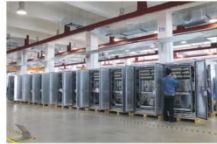
高速动车组电气控制柜生产线 Production line for electric control cabinet of high-speed motor train units
