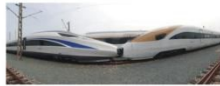
钩缓产品助力中国标准动车组实现双编联 SIF's coupler and draft gear products boosted the double-heading of China's standard motor train units
